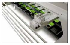
With the hold down beam raised there is enough distance between the ball screws to pull a 1250 mm sheet through (not RAPIDO 13).
