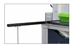
Equip your EVO DUO with a long squaring arm (up to three meters), and add one or more T-grooves and tilting stops.
