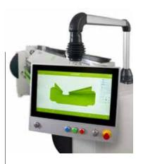
With **ProLink W** you can get precise and fast control of your metal folder. You can choose between using a stored profile, drawing your own custom profile or entering your measurements with classic line-by-line
