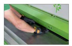
The position of the hold down beam only 32 mm from the cutting line means minimal waste.
