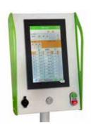
EasyLink is a complete and user-friendly control system for quick and easy programming. EasyLink can store 1000 profiles each with 99 steps. In every program step, the angle, gauge dimension, opening height, clamping pressure and hem pressure can be programmed. Some of the special functions available
