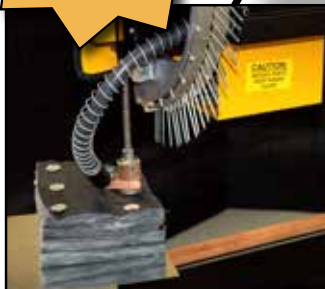
Wider mouth design for welding up to 4" duct liner with 4" weld pins
